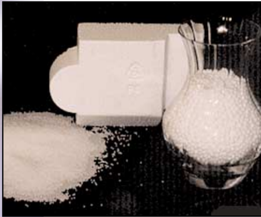
Expanded polystyrene manufacturers use pentane as its primary blowing agent. EPS transport packaging has never been made with CFCs (chlorofluorocarbons) or HCFCs.
